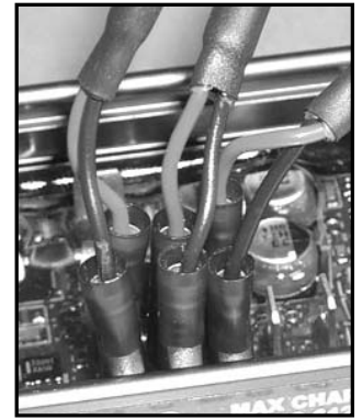
Figure 4 - Proper attachment of optional battery and alternator temp sensors at the regulator.
